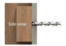
Warning: Do not drill deeper than the thickness of gypsum wallboard (drywall) material.
