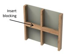
Insert no less than 2"x 4" wood blocking or locate in vertical stud.
