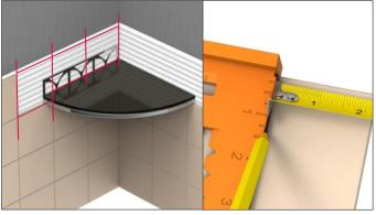
Cut wall tiles to follow corresponding pre-slope, allow 1/16" for grout spacing between wall tile and shelf tile.
