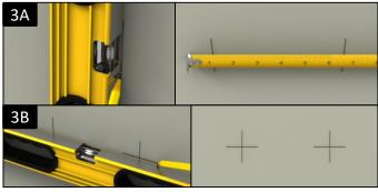
As illustrated in 3A - Use a level to determine position of right spacer and mark a vertical line. Measure precisely 5 1/2" from this line to locate the position of left spacer.
