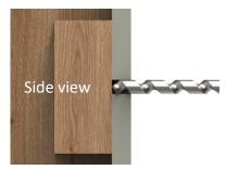
Warning: Do not drill deeper than the thickness of gypsum wallboard (drywall) material.
