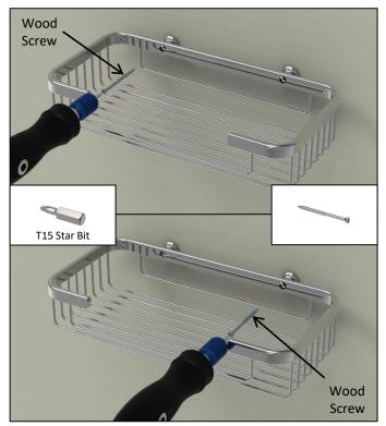
Mount basket with stainless steel wood screws, both left and right sides, with provided star drive bit in kit (or any T15 star drive bit) using a multi-bit screwdriver or power drill.
